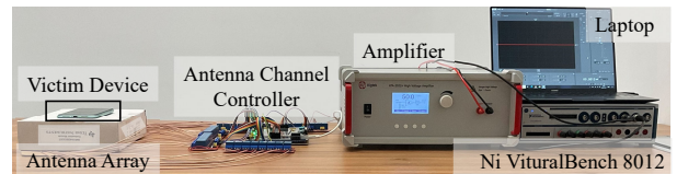
Fig. 7. Prototype of the designed attacking device.
