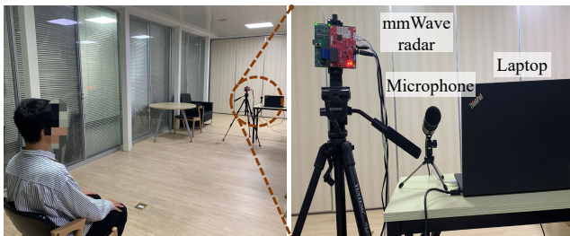
Figure 6: Experimental setup. A mmWave radar and a microphone receive signals from subjects sitting 7 meters away.
